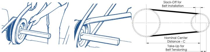
6. The nominal center distance should be determined from a standard pitch length and designed so that the centers can be moved closer together and farther apart to allow for installation and tensioning. The following tables are minimum allowances which allow for manufacturing tolerances as well as stretch and wear of belt. If the drive was designed following the guidelines below, there should be no problem installing or tensioning a belt of the correct length on the drive.
