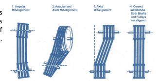
Use a straightedge to check drive alignment. All four points of the straightedge should contact the pulley. Use the straightedge in different positions to check for all kinds of misalignment. In multi-belt drives, misalignment can cause belts that are actually all the same length to appear different lengths. Extreme misalignment can cause rollover and severe belt wear.
