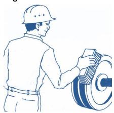
2. Inspect pulleys for wear. Worn pulleys greatly reduce belt life. Extreme wear can lead to belts bottoming in grooves. The result is slippage and excessive heat buildup. Use a pulley groove gauge to check for wear. V-belts should ride at least flush with the top of the pulley and may ride out up to 0.2". Check for burrs, nicks, gouges and severe scratches as these will drastically reduce belt life. Replace if necessary.
