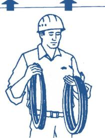
4. Ensure all belts are the same. Do not mix belt brands. Do not mix belt constructions. (Such as raw edge, cogged, wrapped, single and banded) Do not mix new and used belts. The new belt or belts will carry the entire load. Do not mix used belts from different drives. Any mixed belts will cause the load to be carried unevenly, causing the belt carrying the majority of the load to fail rapidly, followed by the remaining belts.
