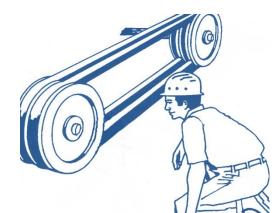
Properly installed belts generally do not require much maintenance. V-Belt drives are recognized as extremely reliable, trouble free and efficient. The main ingredient of good maintenance of a belt drive is to look and listen. Any of the following can be detrimental to belt life but if corrections are made and the belts have not been damaged, the drive will continue to perform well.
